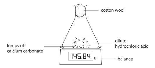
The mass of the flask and contents is measured at regular time intervals.
